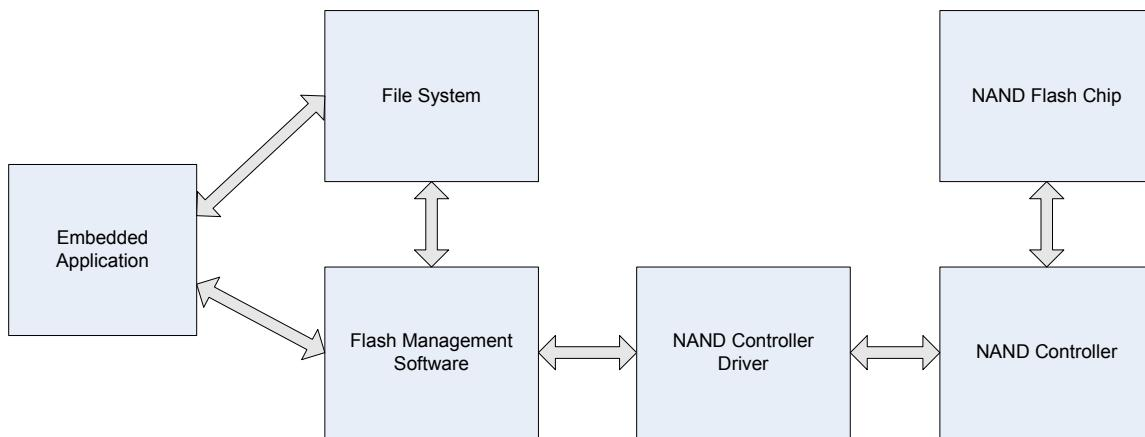
NAND Controllers require specialized software to hide the unpleasant details of the NAND controller and NAND Flash itself and presents the user with a clean and highly usable interface to the memory.
